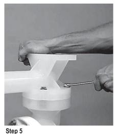
Using a 9/16" wrench, loosen the inlet manifold from the liquid chambers.
