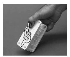
**Step 3**Lift away air valve assembly and remove air valve gasket for inspection. Replace if necessary.
