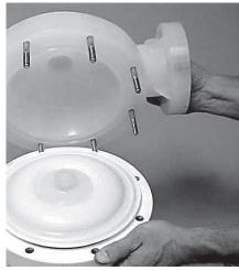
**Step 8**Remove the liquid chamber to expose the diaphragm and outer piston.
